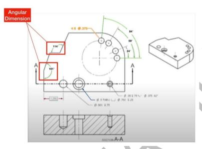
Trainee Action: Touch the angle that is not correctly dimensioned.
