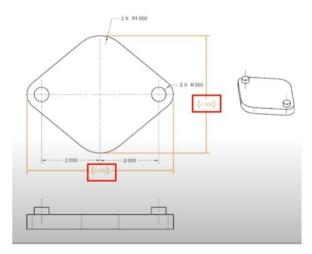
This is called a reference dimension. Using reference dimensions indicate the approximate size of an object. If these dimension values were not in parenthesis this object would be over dimensioning
