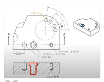
This is further confirmed by the cross section shown below the drawing.
