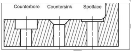
Earlier we covered the symbols couterbore and countersink, mentioned their relationship to two types of screws. Let's dive deeper into types of screws and how to read annotations specific to this tool.
