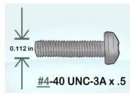
The number four is the thread diameter. [highlight 4] Along the shaft of the screw are tiny grooves, these grooves are what is being measured in diameter.
