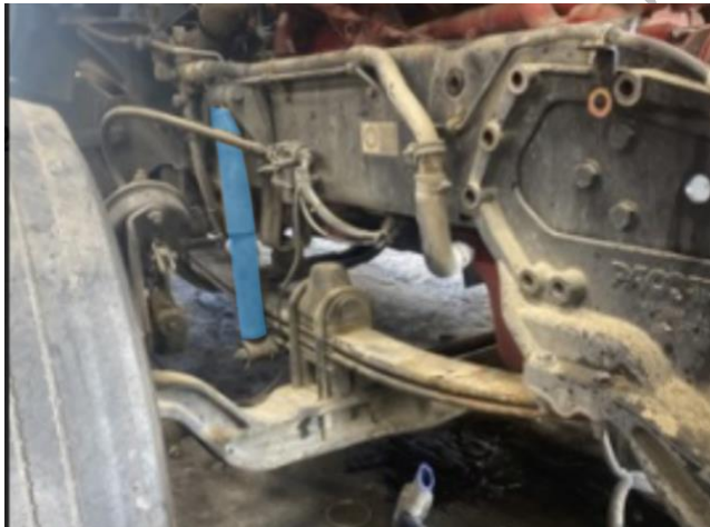
[shock absorber installed (front passenger side)]
