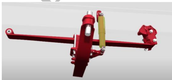
[front shock absorber installed]
