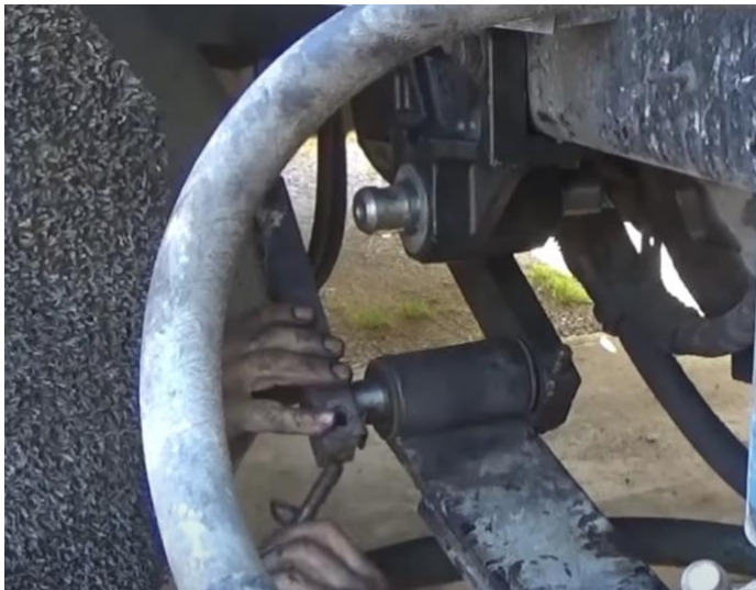
[shackle being placed installed on end spring pin]
