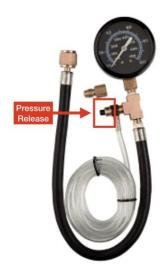
Keep your eye on the count down. At the 15 second mark, touch the pressure release button again to shut off the flow of fuel.
