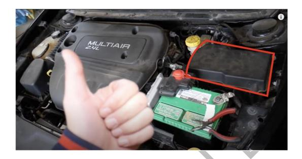
We need to take off the fuse box cover to find out where the relay and fuel pressure fuse are located.
