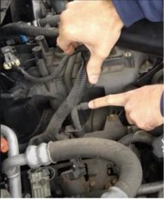
Twist once to loosen the cap on the Schrader valve.
