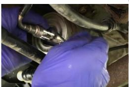
Now the line needs to slide off. There may be some fuel that leaks out. I've put a bucket on your cart and positioned it under the fuel line to catch any residual fuel.
