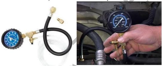
On the cart, grab the valve at the end of the pressure gauge.
