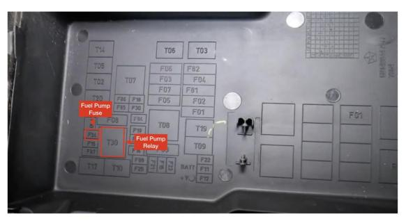
Let's remove the relay and fuel fuse from the fuse box one at a time. Use the grip button on your controller to remove the relay.
