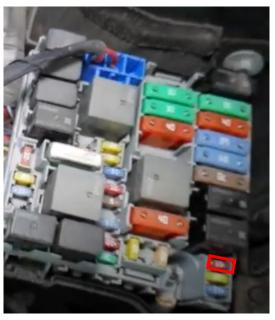
On your cart is a tool called a fuse puller [highlight] that will help you remove the fuses [highlight airbag fuses].
