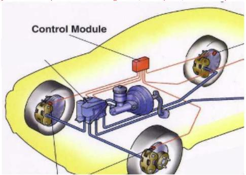
ABS allows the driver to steer during emergency braking and allows the vehicle to stop at a shorter distance on low traction surface. Let's put the wheels in motion so we can see it happen. [all four tires begin to rotate at the same speed]
