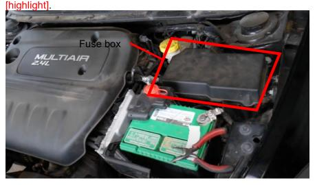
We need to take off the fuse box cover to find out where the airbag fuses are.
