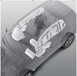
Some common locations in a car are the driver's side airbag [highlight], steering wheel airbag [highlight], the passenger side airbag [highlight], and curtain airbags [highlight]. There may be additional airbags depending on the manufacturer.
