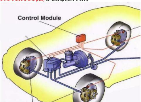
This allows the wheels to spin intermittently and regain traction during braking, causing the pulsating fee [animate tire pulsating while simultaneously pulsing the oculus controllers]. ABS allows a driver to maintain control of the vehicle during emergency braking by decreasing the time to stop and by steering around obstacles while braking.
